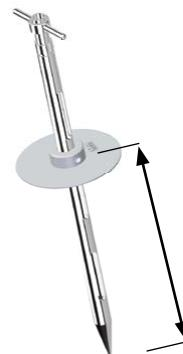
3. Fix with an Allen key (5 mm) (not included in the scope of delivery). Use the Allen key only for fixing and loosening, remove again after use.
