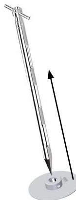
2. Position the depth stop at the desired height on the sampler.
